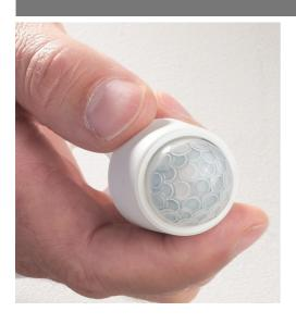
The EBR-MINPIR presence detector is designed to provide automatic control of lighting via the RAPID or LMS lighting control systems. It detects movement using a PIR sensor to turn the load on. When an area is no longer occupied the load will switch off after an adjustable time out period.
